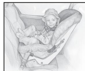
Figure 2. Convertible car safety seat used rear-facing.
